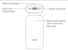
The battery level check button is not a power button.
